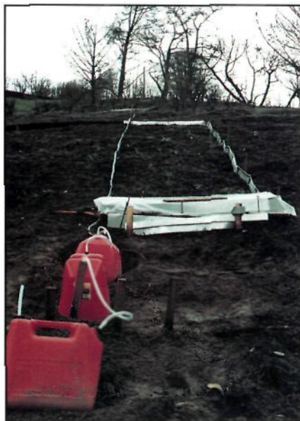
Photo 3. A runoff and erosion plot. Runoff is funneled from the trough to 5-gallon plastic containers connected in series to store runoff and suspended sediment. The emergent vegetation is Indian Soap Plant ( Chloragalum pomeridianum ) and is not a result of the reseeding effort.
