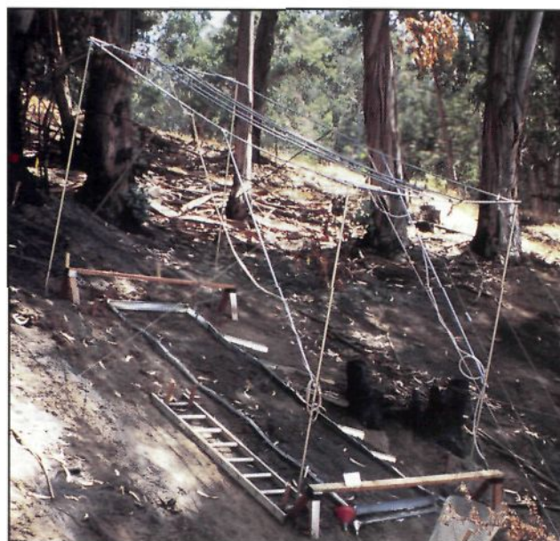
Photo 4. The simulated greater-than-100-year storm was applied by rapidly moving two nozzles on trolleys suspended from central rails in the tubular frame 10 feet (3 m) above the plot. Runoff and sediment were collected from two troughs, an upper trough to monitor overland flow, and a lower trough to monitor flow through the wettable soil layer.
