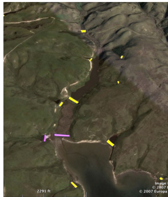
Figure 3: Big and Little Limantour watersheds (left to right) showing mainstem and major tributary dams. Pink dams are breached.
