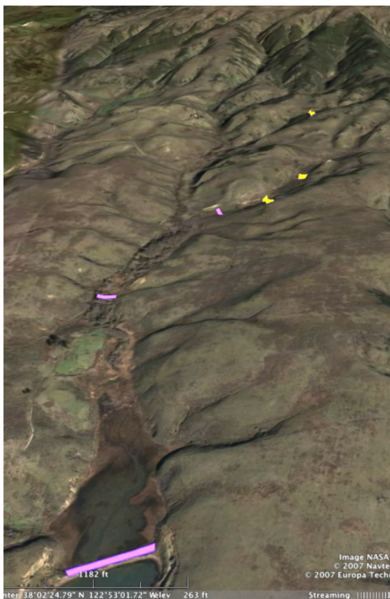
Figure 4: Glenbrook watershed showing mainstem and major tributary dams (pink dams are breached). The lowermost mainstem dam was breached in the historic January 1982 storm.
