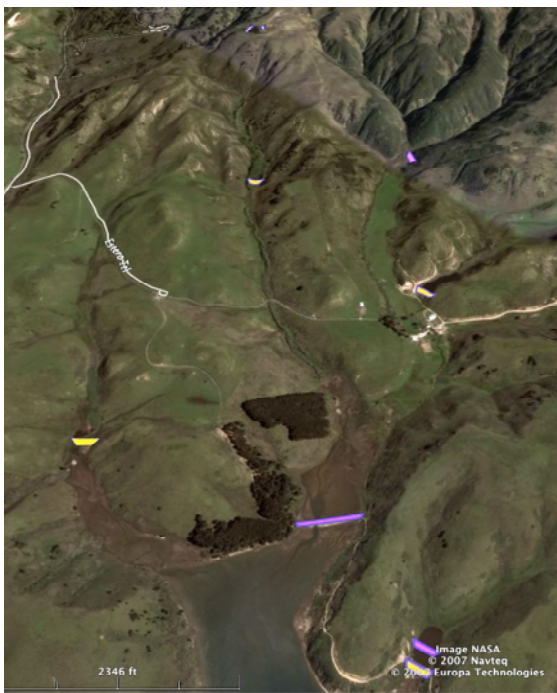
Figure 2: West Home, East Home, and Home Ranch watersheds (left to right) showing mainstem dams. Pink dams are breached.
