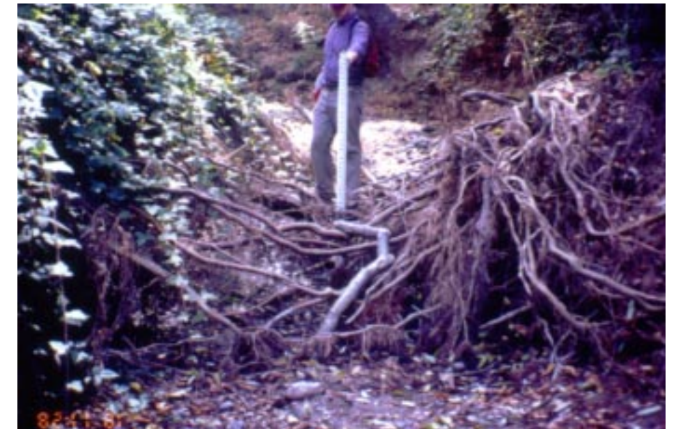
(Photo 58) Exposed roots in 1996 indicate the amount of bed incision that has occurred since 1987 when this reach was previously surveyed.
