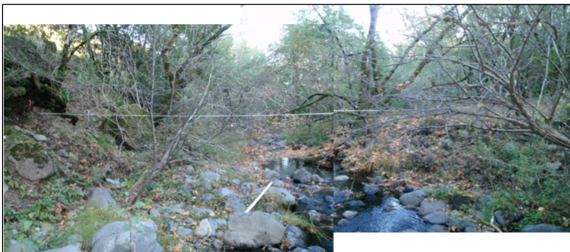
Figure 57. Station 20,405 ft on the Carriger Creek alluvial fan is shown looking downstream at the Upper Cross Section. Notice the 10-ft-high terrace on the right bank. It indicates long-term incision at the site. Photo by L. Collins Dec 2011.
