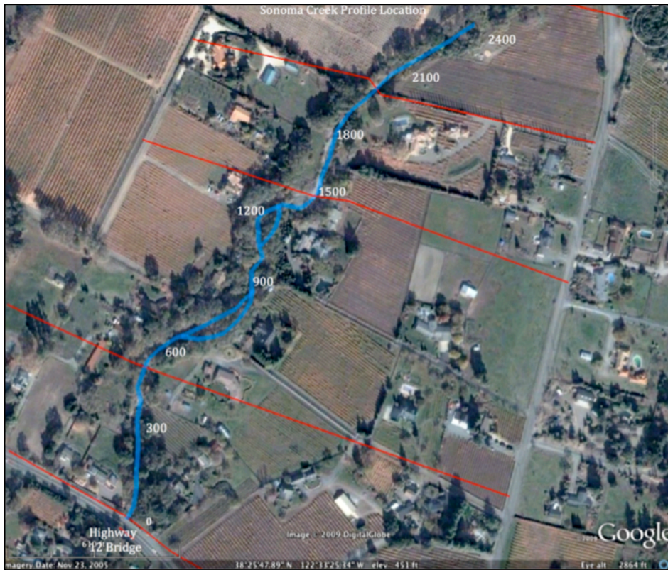
Figure 12. Distance station locations are shown in white along Sonoma Creek upstream of the Highway 12 Bridge. Its two major channel braids are also shown. They are active channels at flows less than bankfull discharge. Red lines indicate cross section sites previously surveyed by PWA (2010). Map source: (Sec 2010).
